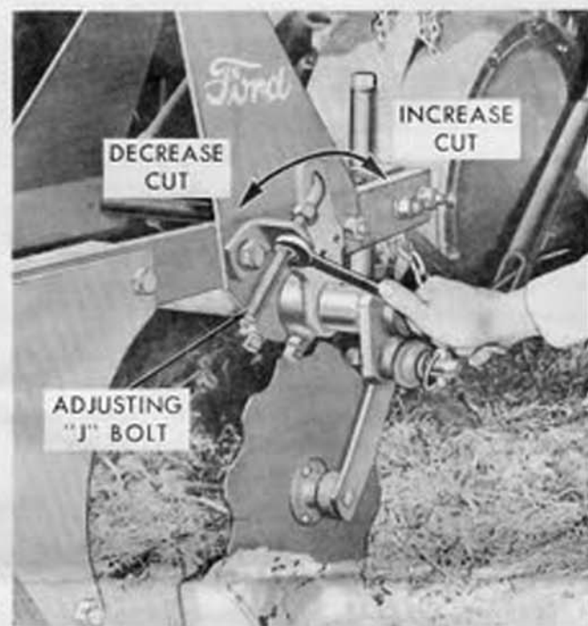
Figure 8 - Changing Width of Cut
